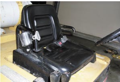
Wear a seat belt to keep you inside if your forklift overturns.
