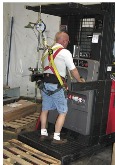
The operator of an order picker type forklift must wear a safety harness to protect against the fall hazard at an elevated location.
